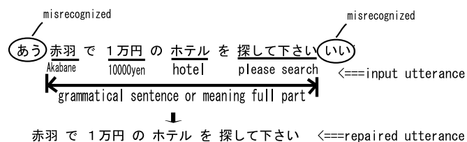
Figure 3: An example of removing recognition error caused by logging error.
